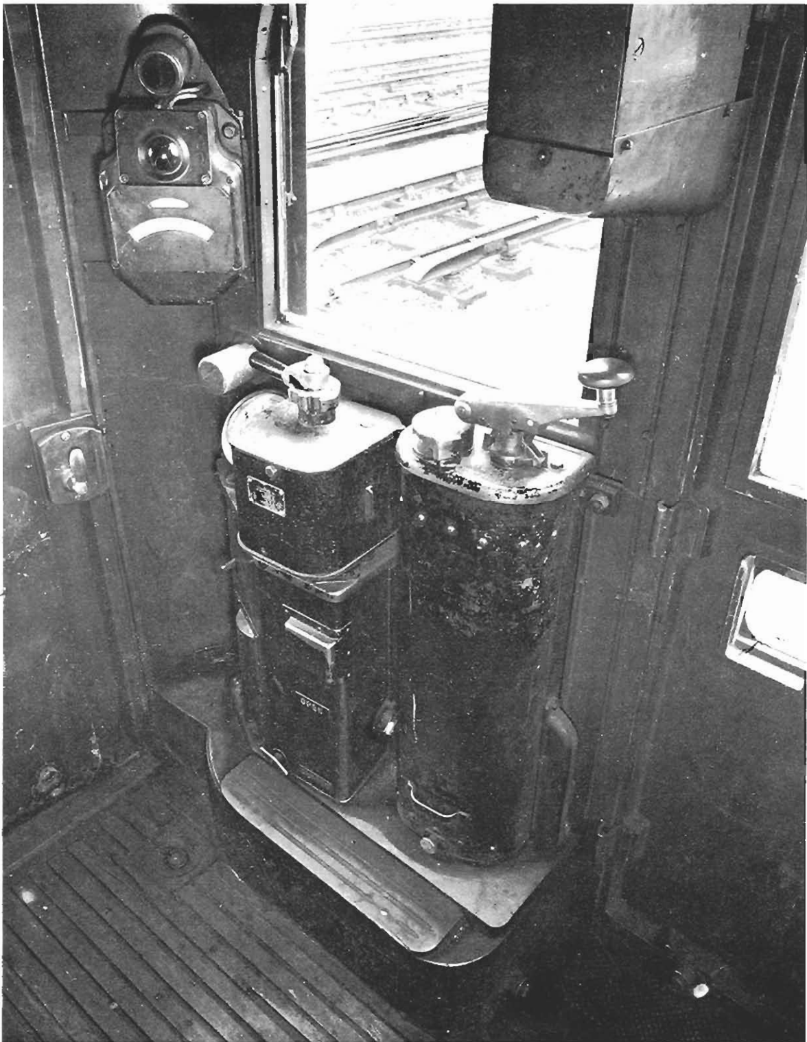
Photograph 3. Driver's Cab of 1938 Tube Stock, showing, on the left, the Driver's brake handle and, on the right, the Master Controller with the Deadman's handle. (By Courtesy of London Transport)
