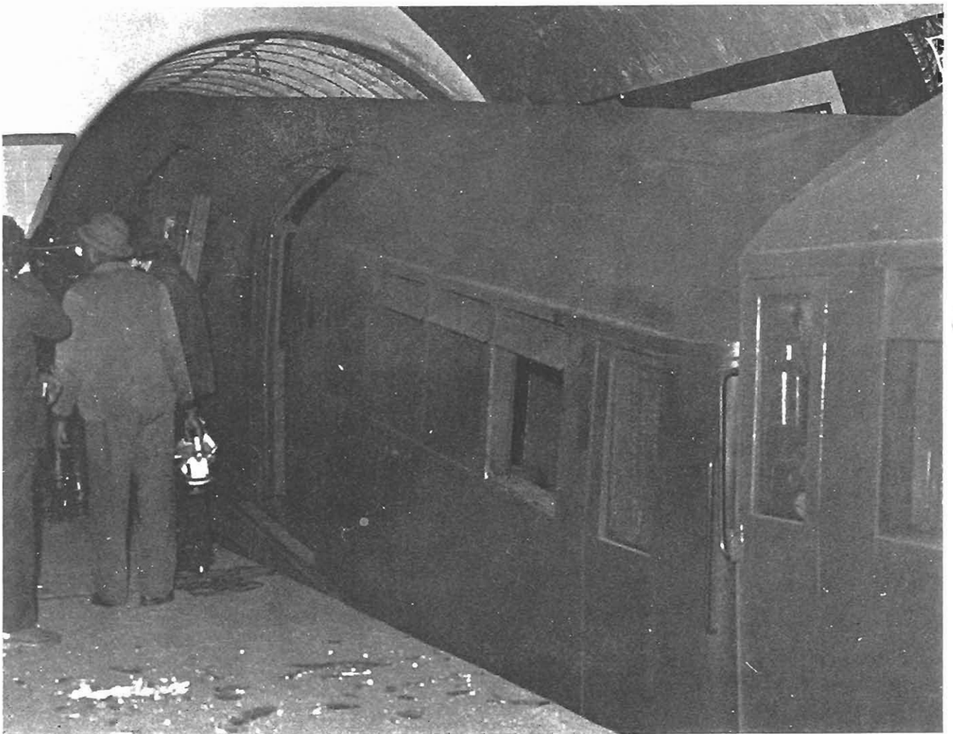
Photograph 5. Wrecked train showing position of third car. (By courtesy of City of London Police)
